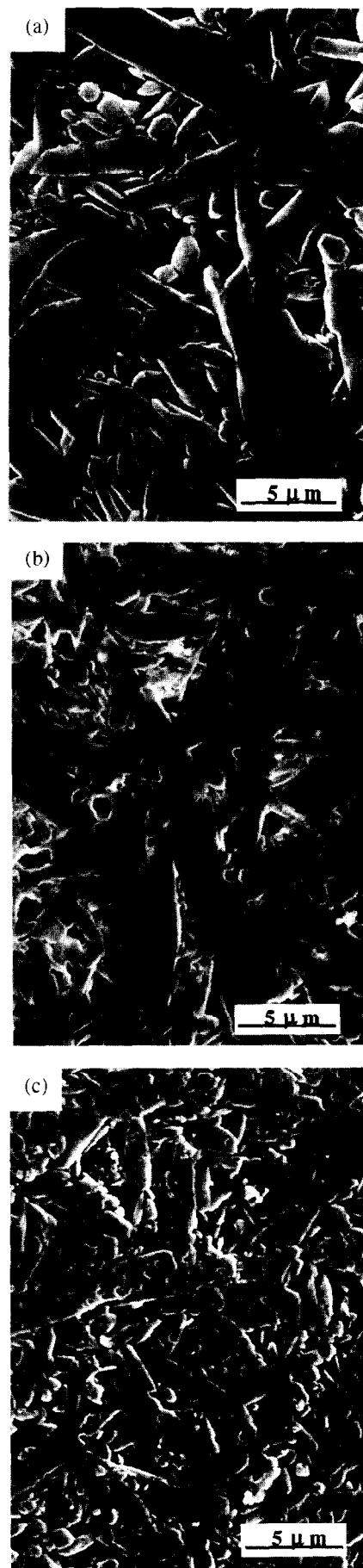
Fig. 1. SEM micrographs of \text{Si}_3\text{N}_4 containing (A) 0 vol%, (B) 5 vol%, and (C) 20 vol% of SiC nanoparticles. All the specimens were hot-pressed with 14 wt% of \text{Yb}_2\text{O}_3 at 1800^\circ\text{C} for 2 h.
